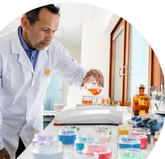
Pouring candles in the application technology to check the stability of fragrance components in wax.
